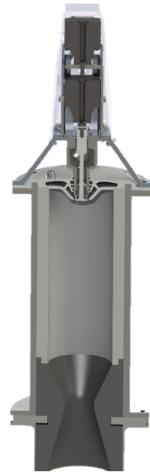
Figure 16 : Ground design of the thrust modulation pintle
