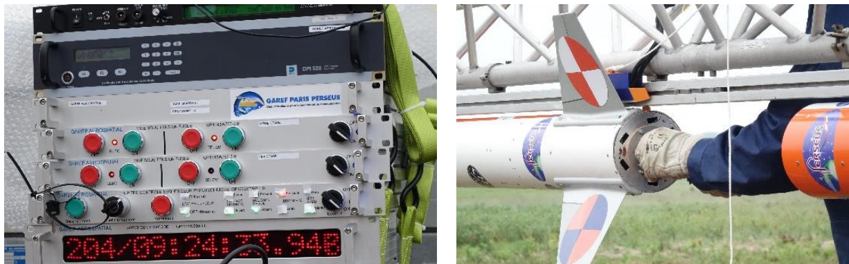
Figure 6: Ground segment for the pyrotechnic sequencer and installation of the igniter by the pyrotechnician
