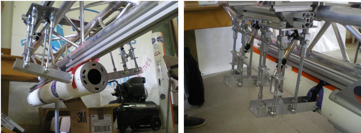
Figure 14: The Two-staged Rocket Manipulation System under test
