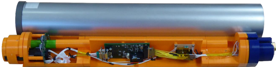
Figure 5: Dummy motor in opened configuration, with the casing and the main half of the 3D-printed assembly
