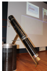
Figure 7: Tank, combustion chamber and nozzle – PEGASE
