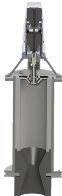
Figure 16 : Ground design of the thrust modulation pintle
