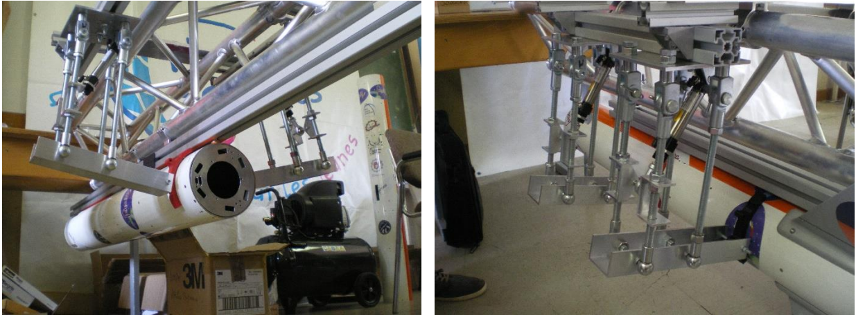
Figure 14: The Two-staged Rocket Manipulation System under test
