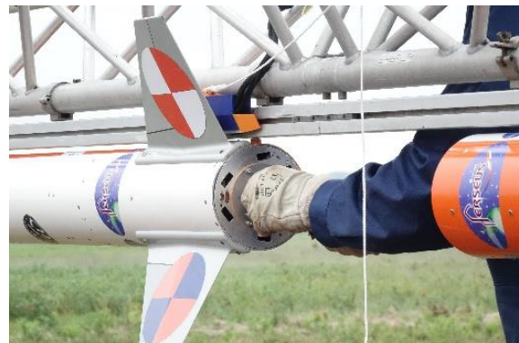
Figure 6: Ground segment for the pyrotechnic sequencer and installation of the igniter by the pyrotechnician
