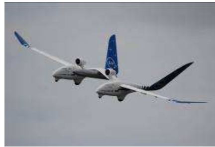
Figure 10: Remote controlled model probationary of EOLE – 1/2.2 scale
