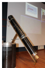
Figure 7: Tank, combustion chamber and nozzle – PEGASE
