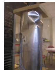
Figure 8: Buckling tank - ENSICA
