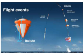
Figure 26: Ballute and hemispherical Systems Concept
