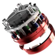
Figure 20: ASTREOS 1 Separation and recovery device
