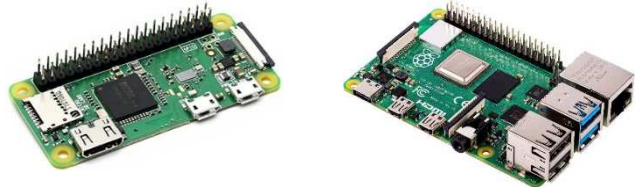
Figure 19: ASTREOS 1 Raspberry Pi4 and Pi0
