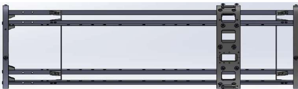
Figure 13: SERA4 avionic section skeleton
